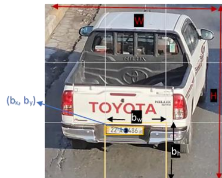
Fig. 5. LP detection using YOLO with 3x3 grid cells.
