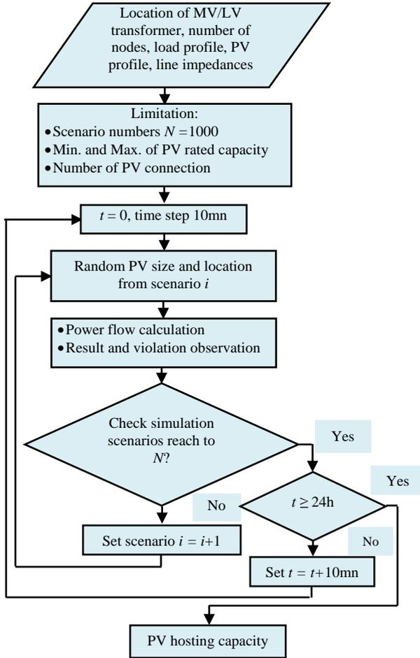
Fig. 4. Flow chart of PV hosting determination.
