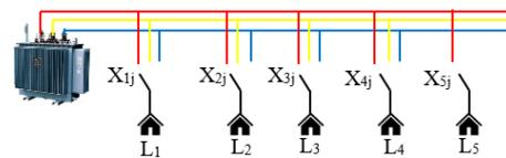
Fig. 3. Load connection to any phase by switch  $X$ .
