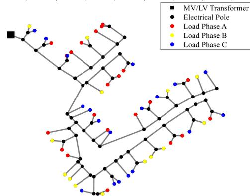
Fig. 10. Topology of test system by phase balancing on load profile.
