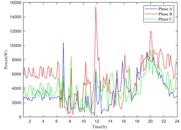
Fig. 9. Load profile of each phase of scenario 2.
