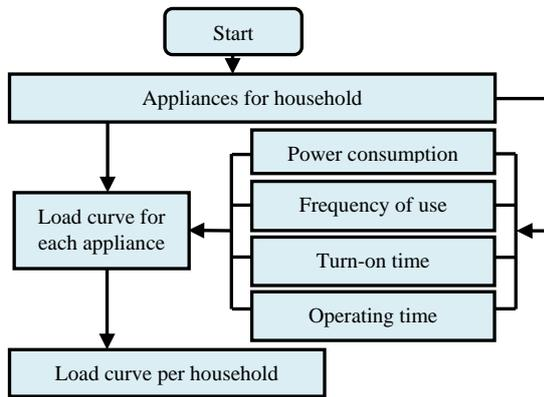
Fig. 1. Procedure of load profile simulation.
