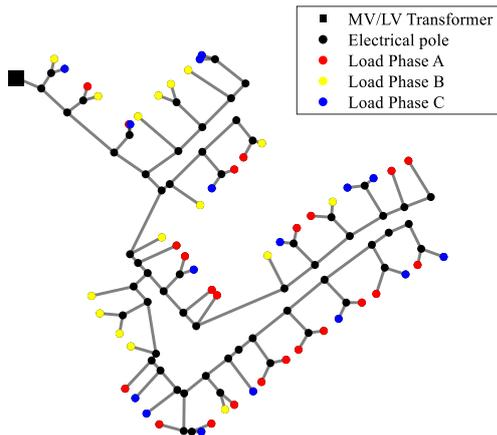
Fig. 8. Topology of test system by phase balancing on peak power.
